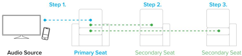
**Step 1:** Power on just the primary seat of the lounge suite by pressing the Pwr/Vol dial for 3 seconds. It will automatically enter Bluetooth pairing mode and the LED lights around the Power/Volume dial will be flashing.
